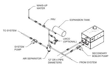
FIG. 36 Primary/Secondary Piping of a Single Boiler
